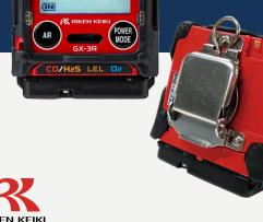
The GX-3R provides 3 preset alarm settings per gas plus an additional alarm for a higher detection range. The GX-3R internal data logger allows 3600 event logs and 300 hours which can be read out using an IrDA link. A loud 95dB alarms buzzer is also a built-in feature.
